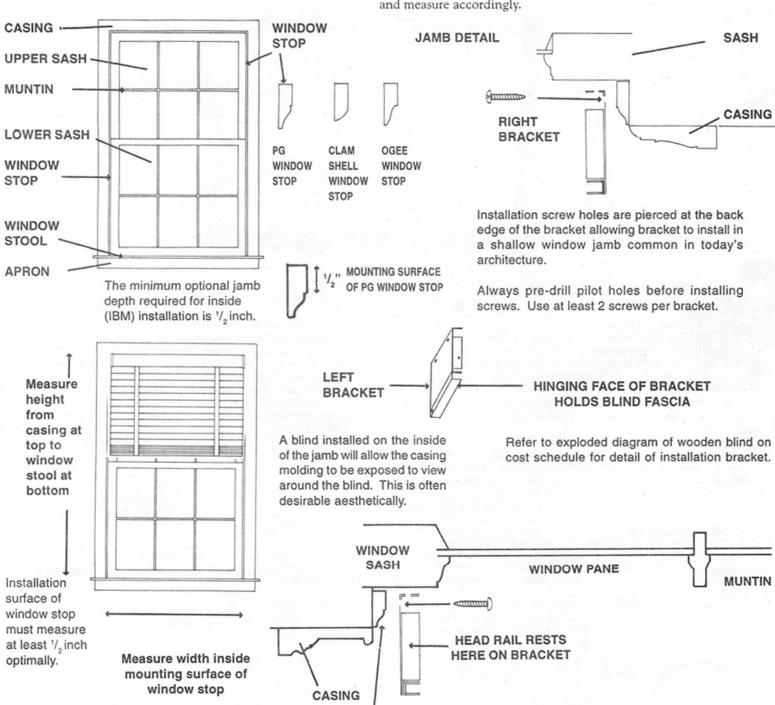
PG WINDOW STOP. This is the mounting surface. The bracket will install at this point.
